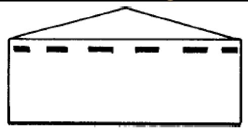
• Incorporate a fixed cone shaped roof with inner floating roof.
